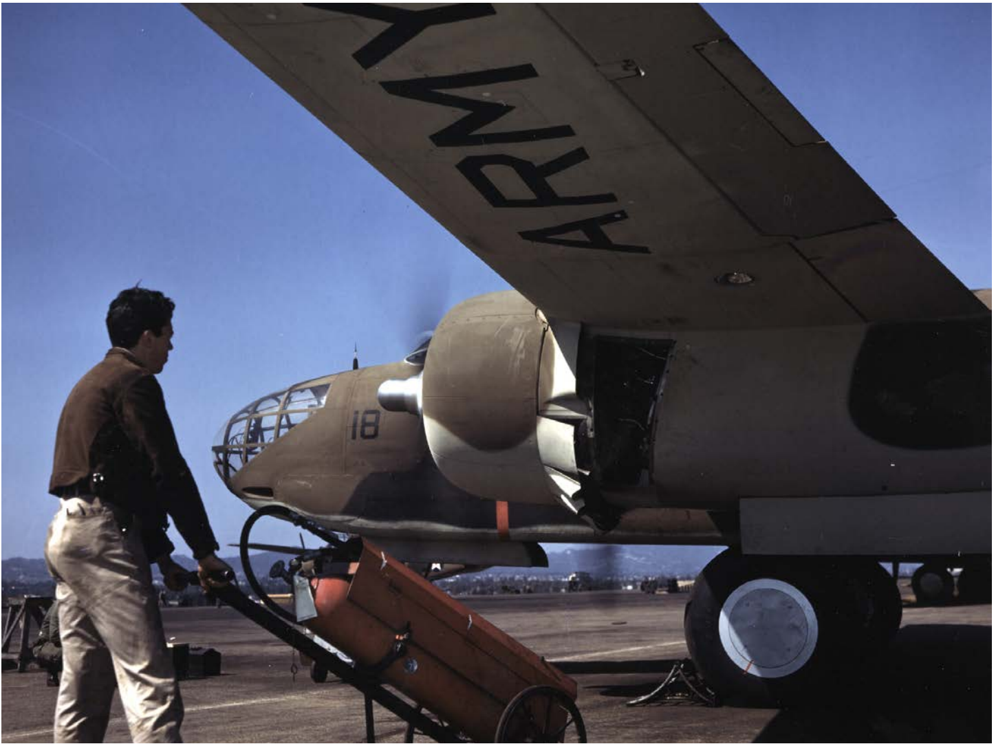
Another view of DB-7C D-6282 in May 1942 on the ramp at Douglas during engine runs. These aircraft were painted in accordance to the British DB-7B scheme. The primary difference between the RAF DB-7Bs and the MLD DB-7Cs was the provision to carry the U.S. Mark XIII torpedo, as the MLD planned to use their 48 DB-7Cs as torpedo bombers. (Douglas)
